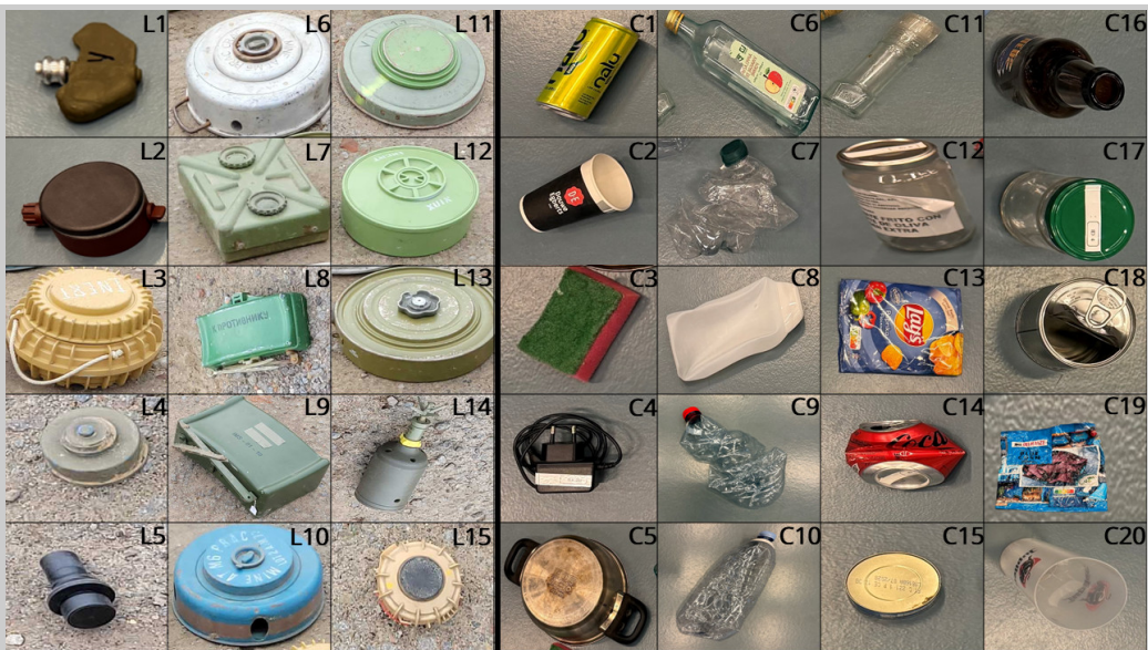
Fig. 2. Overview of all the objects included in the dataset. The objects on the left side of the black line are landmines (L) , while the objects on the right side of the black line are common items (C) . For what concerns the landmines (L) - L1 : PFM-1 “Butterfly”, L2 : PMN, L3 : TC-3.6, L4 : M35, L5 : C-3 “Elsie”, L6 : M6 (grey), L7 : TMA-2, L8 : MON-50, L9 : MON-90, L10 : M6 (blue), L11 : TMM-1, L12 : Type 72 (P), L13 : TM-46, L14 : PROM-1, L15 : VS-50. For what concerns the common items (C) - C1 : Soda metal can, C2 : Disposable paper cup, C3 : Sponge, C4 : Plastic charger, C5 : Metal pot, C6 : Glass vinegar bottle, C7 : Plastic water bottle (significantly crumpled), C8 : Plastic shampoo bottle, C9 : Plastic water bottle (partially crumpled), C10 : Plastic water bottle (slightly crumpled), C11 : Glass pepper dispenser, C12 : Glass jar (grey cover), C13 : Plastic chips bag (slightly crumpled), C14 : Metal coke can, C15 : Metal tuna can, C16 : Glass beer bottle, C17 : Glass jar (green cover), C18 : Metal corn tin, C19 : Plastic chips bag (significantly crumpled), C20 : Plastic cup.
