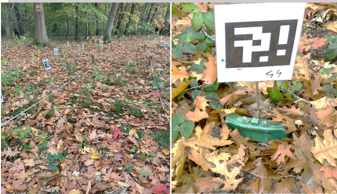
Fig. 5. Left - The track is ready to sample the reference sequence. Right - A MON-50 landmine and its corresponding AprilTag. The pose of each AprilTag, denoted as A_i , is evaluated, allowing determination of the position of the corresponding target T_i .
