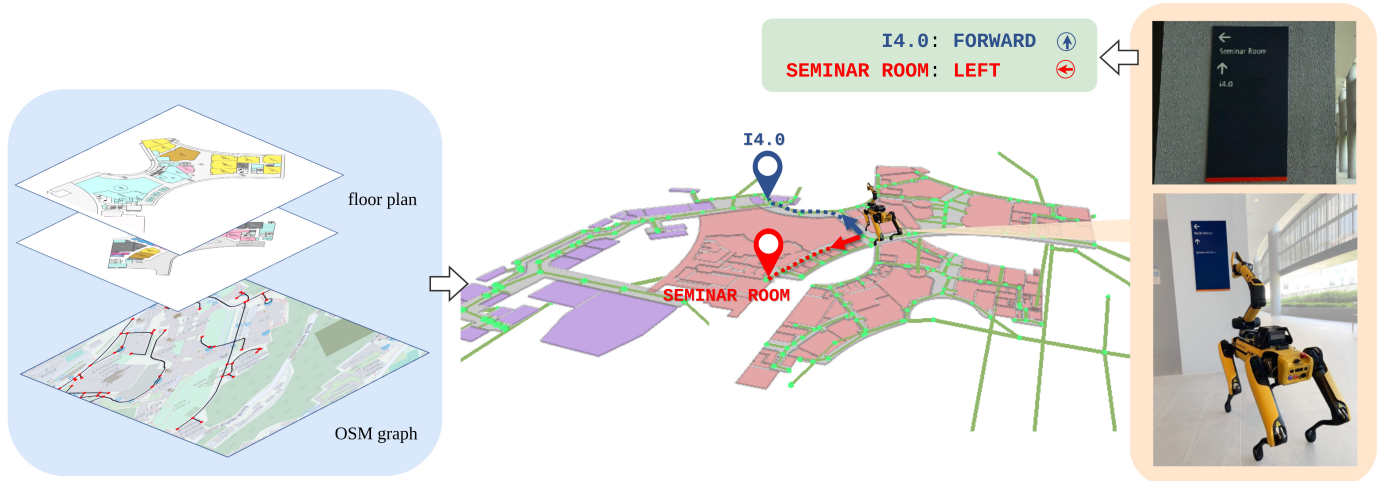
Fig. 1: Global localization using SignLoc with a Boston Dynamics Spot robot. The robot detects navigational signs and extracts directional and locational cues. To localize, it matches these cues to a large-scale, indoor-outdoor navigation graph, constructed from publicly available maps.
