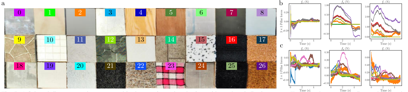
Fig. 5: a) Selected diverse natural textures used in the experimental evaluation, with numbers indicating texture IDs and colors corresponding to those used in the feature analysis figure. Illustration of raw tactile observations for Texture ID 0 (in b) and Texture ID 26 (in c) under same action parameters during the vibrosliding (vibration+sliding) interaction, demonstrating the distinct and information-rich tactile signals.
