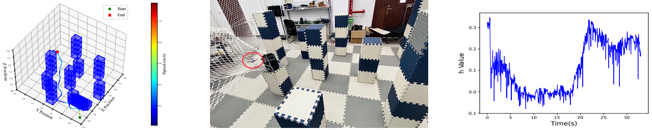
Fig. 5: Real-world experimental results of the 3D-UAV System. For (a), the visualization of experiment, blue squares represent the obstacle region, and the color variations along the trajectory indicate the robot's speed. For (b), the scene of the experiment. For (c), the value of h remains non-negative except for several short intervals.
