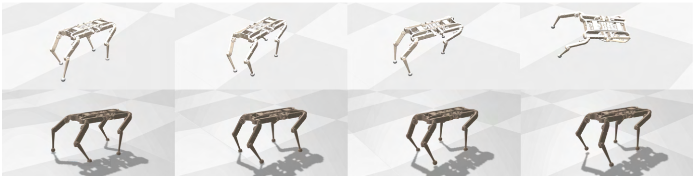
Fig. 6. Comparison on inclined terrain outside the training distribution between PPO ( top ) and TD-CD-MPPI ( bottom ), both using a lower-bound constraint on foot air time as gait shaping constraint. The policy trained with PPO becomes unstable under the out-of-distribution conditions, while TD-CD-MPPI keeps consistent locomotion behavior.
