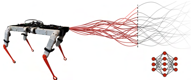
Fig. 1. The proposed TD-CD-MPPI controller enables the use of reduced control horizons by using a learned terminal value function to approximate long-term returns.
