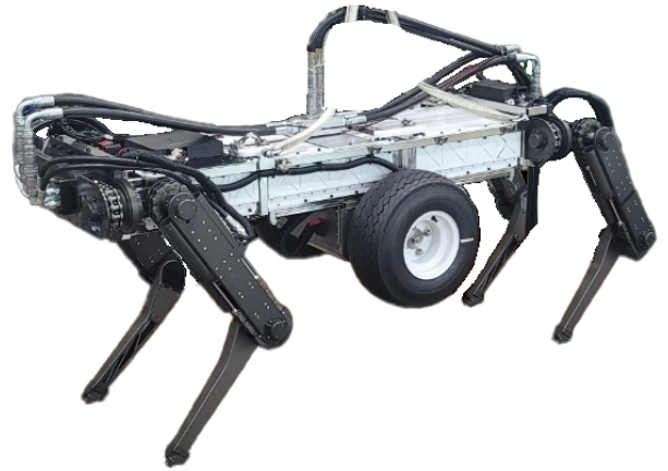
Fig. 2. BeTheX-Q, a hybrid-locomotion platform combined with wheeled & quadruped system
