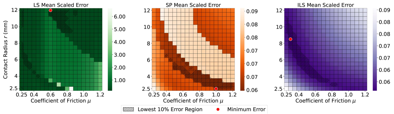
Fig. 15. Landing pose error heatmaps for the three models: “LS,” “SP,” and “ILS.” The heatmaps show the mean scaled landing error (39) as a function of contact friction coefficient \mu and contact radius r . Darker colors indicate lower errors. The hatched region highlights the lowest 10% of landing errors across the parameter space. The red marker indicates the optimal contact parameter for each model.
