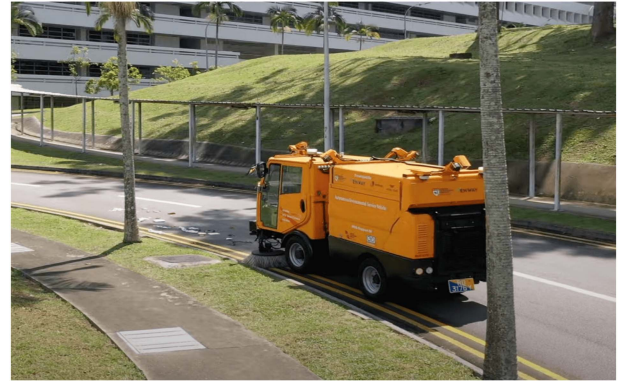
Fig. 1. Illustration of curb following in road sweeping applications. [The autonomous vehicle is required to maintain a specified lateral offset while following the curb to perform road sweeping tasks.]
