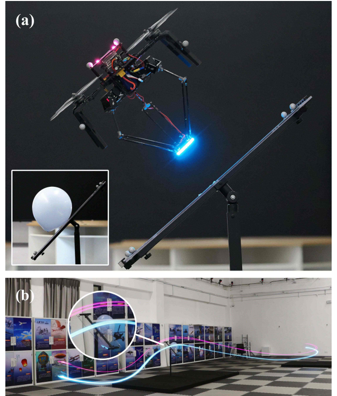
Fig. 1. Demonstration of aerial striking using whole-body integrated motion planning. (a) The aerial manipulator executes a planned trajectory to reach a constrained waypoint, maintaining an attitude parallel to the inclined plane while configuring its delta arm for balloon striking. (b) Time-lapse visualization capturing the complete execution of the planned motion.
