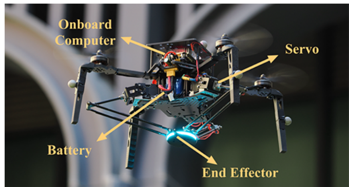
Fig. 13. Real-world aerial manipulator platform used for validation.
