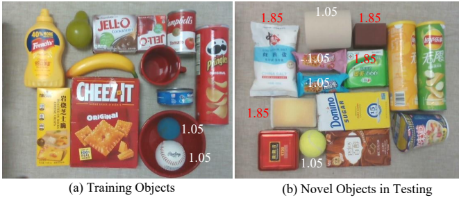
Fig. 6. (a) Objects adopted in training scenarios. (b) Novel objects in testing where some of them are from unseen classes. Numbers beside objects mean the deformability coefficients, and those without numbers are rigid objects.
