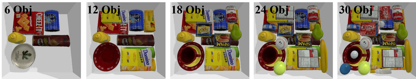
Fig. 9. Visualization of the generated packing plan including the object sequence, orientation and location in the packing box. Our method learns effective packing policies such as putting cups on plates and placing balls in cups to enhance the space utilization ratio.
