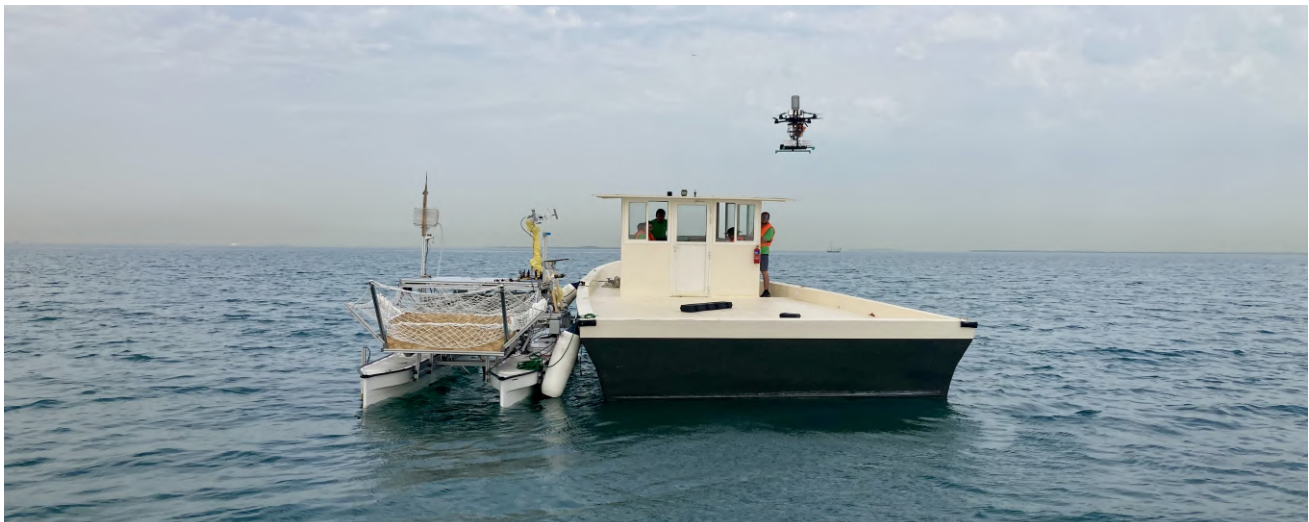
Fig. 1: ASV-UAV robotic team in an object pickup task during the MBZIRC competition. The ASV is docked to the target vessel, and a UAV is scanning the deck of the target vessel in search of target objects. The robotic arm onboard the ASV (yellow) tracks and localizes the UAV using the LiDAR attached to its end effector.
