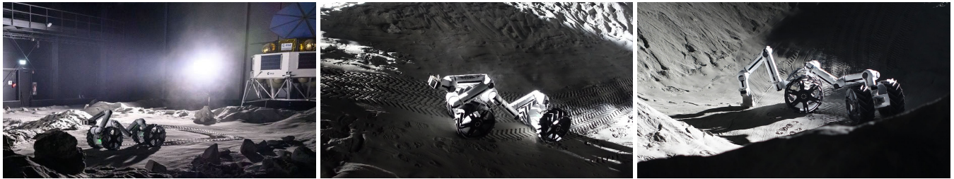
FIGURE 23. Additional field testing on a terrain fully covered with regolith simulant. The MoonBot was deployed in a lunar dust environment and teleoperated to traverse the 20 x 35 m field (left). MoonBot in the Dragon configuration was able to climb a crater with a 20° inclination (middle). The Dragon configuration interacting with a medium-sized rock at the bottom of the crater (right). Unlike silica sand, fine regolith particles were easily lofted by wheel rotation, adhering to and contaminating the robot's surface.
