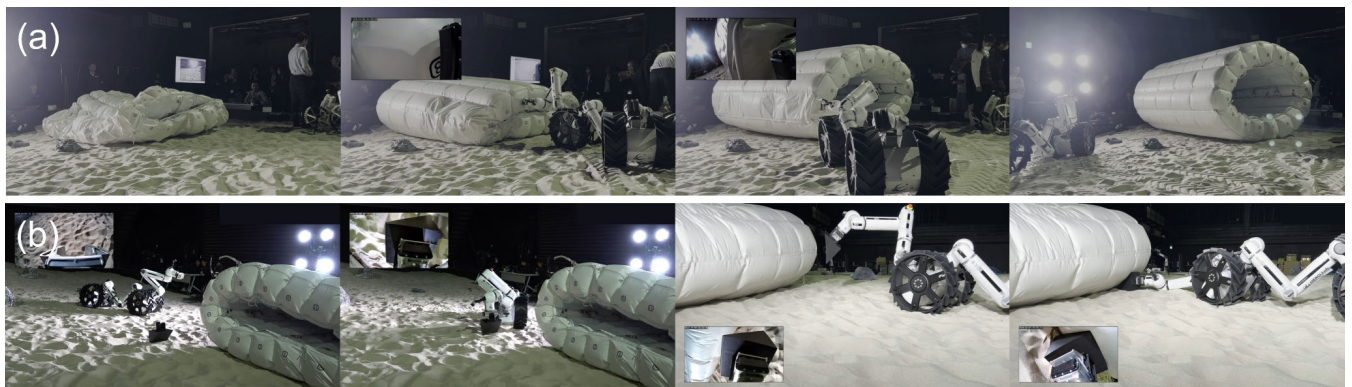
FIGURE 22. Inflatable module deployment assistance demonstration by MoonBot. (a) MoonBot in Dragon configuration monitored the inflation of the module on a cell-by-cell basis using a hand-eye camera. By applying additional pressure to each cell with an external robot, the system verified the absence of gas leaks through internal pressure sensors integrated into each cell. (b) Once the inflatable module had been fully deployed and well-positioned, the robot placed stopper objects to further enhance its stability.
