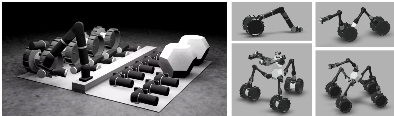
FIGURE 2. Self-assembly of the modular robot concept on the Moon. The robots are transported to the lunar surface as compact modules affixed to the specialized plate called a launch-lock palette, which is housed in the payload space of the landing vehicle (left). Each module is categorized based on its functionality: bases, limbs, wheels, and tool-changing end effectors. Upon arrival, the robot modules can autonomously reconfigure themselves into various morphologies, adapting to different tasks and mobility requirements (right).
