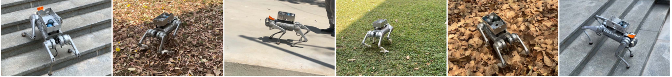
Fig. 1. Hardware deployment of our framework across diverse terrains, including dynamic payload variations on flat ground, slopes, and uneven surfaces, as well as moving payloads (e.g., rolling balls) on stairs. All results are obtained using a single policy, without sim-to-real changes or real-world fine-tuning.
