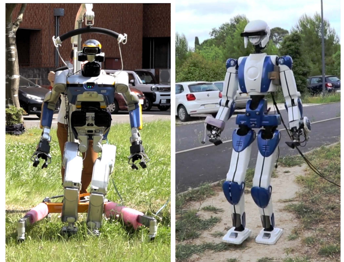
Fig. 19. HRP-2KAI and HRP-4 robots walking outdoors. Experiments with the HRP-4 are done without safety ropes.
