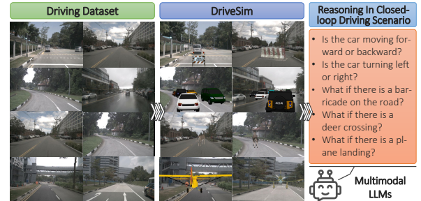
Fig. 1. Are MLLMs world models for driving? We investigate their effectiveness in understanding and reasoning about dynamic driving scenarios from sequential images with an introduced real-world driving and re-simulated dataset. Our experiments show that MLLMs struggle to form coherent narratives, failing to reason about car motion, traffic, etc.
