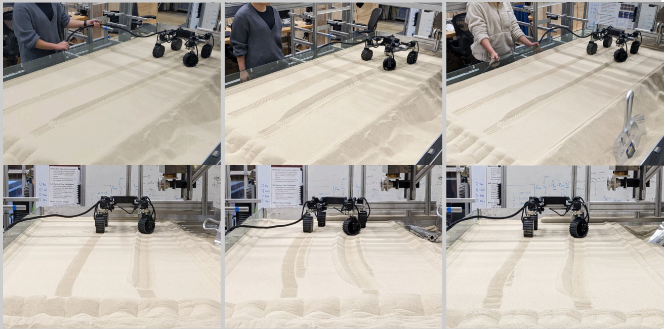
FIGURE 26: Mini rover driving with a stuck steering motor. From left to right: driving without compensation, feedforward with no feedback control, feedforward with optimal feedback control.
