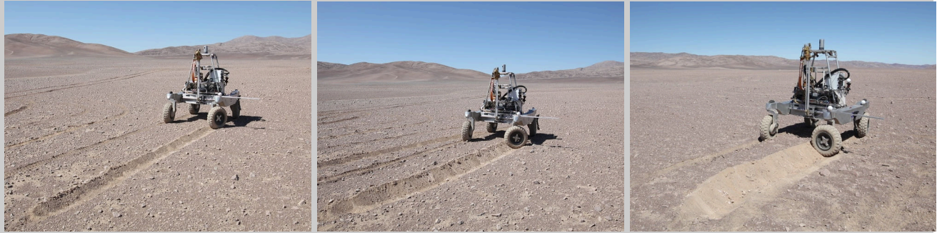
FIGURE 15: KREX-2 driving with a stuck steer motor in the Atacama Desert with hand-tuned compensation. The rear right wheel is stuck at 30° (left), 60° (center), and 90° (right).
