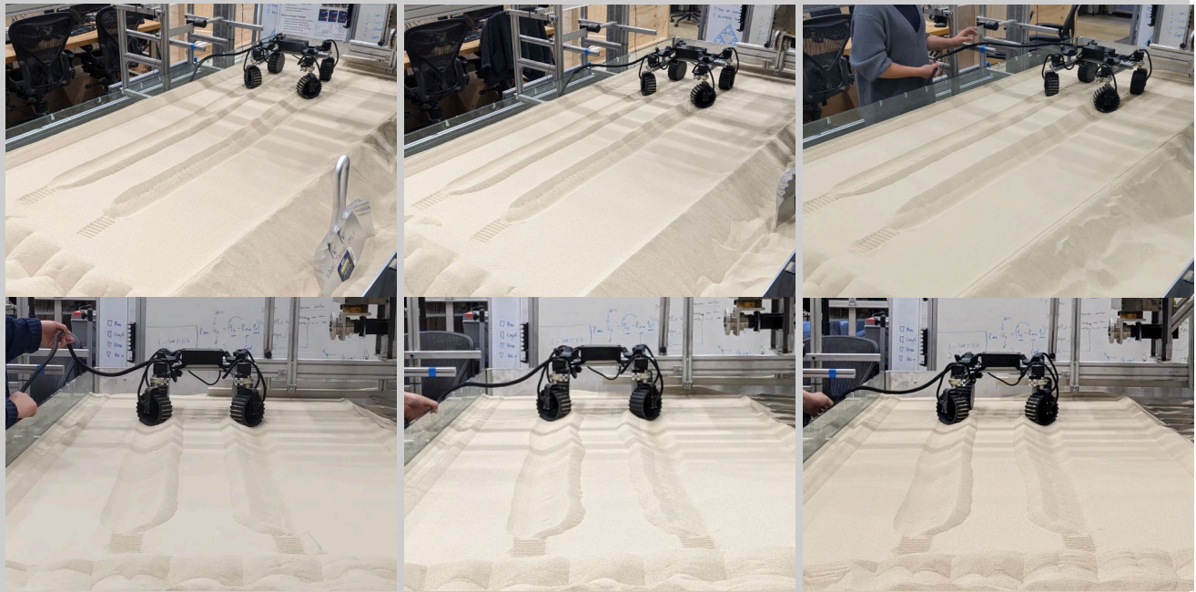
FIGURE 21: Mini rover digging a trench with several driving strategies. From left to right: feedforward trenching primitive only, feedforward with nominal feedback control, feedforward with optimal feedback control.
