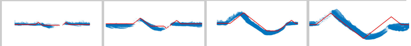
FIGURE 4: LIDAR scans of trenches dug by the KREX-2 rover in the Atacama Desert (blue) overlaid with predicted trench shape (red). The wheel angle for each trench, from left to right, was 0°, 30°, 60°, and 90°.
