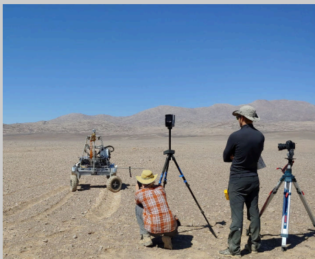
FIGURE 2: Setup of trenching experiments in the Atacama Desert. The KREX-2 rover (left) was driven over unprepared soil, with the FARO ® LIDAR (center) scanning before and after and video recording of each test (right). Not pictured is the Leica Total Station used to track the rover’s position and speed during testing [33].
