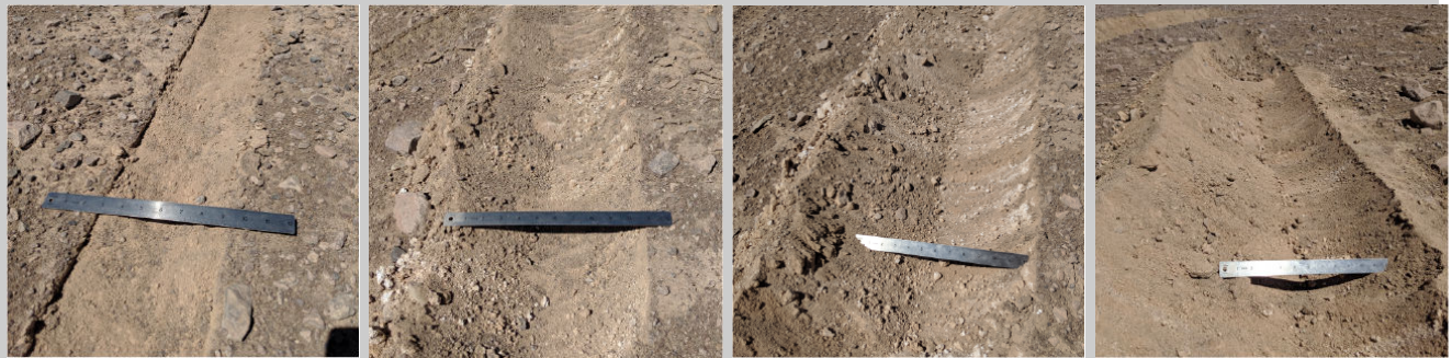
FIGURE 3: Trenches dug by KREX-2 in the Atacama Desert with 1 foot ruler for scale. The wheel angle for each trench, from left to right, was 0°, 30°, 60°, and 90°.
