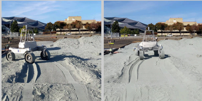
FIGURE 16: KREX-2 rover driving with a stuck drive motor without compensation (left) and with open-loop compensation (right).
