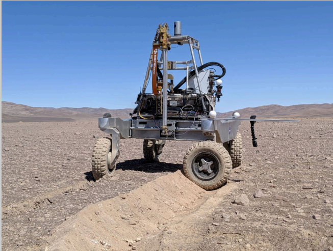
FIGURE 1: The KREX-2 rover after digging a trench in unprepared soil in the Atacama Desert. This trench was dug with the rover speed at 20 cm/s, the digging wheel rotated 90° from the direction of travel, and the digging wheel’s speed at 50 cm/s. The white streaks present in the rover’s track are due to halites in the soil.
