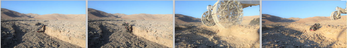
FIGURE 8: Images from a video of KREX-2 helping MiniRHex traverse a natural step in terrain due to water flow in the Atacama Desert. Left to right: MiniRHex tries to climb the step; but is unable to and flips over; once KREX-2 crushes a ramp into the step; MiniRHex is able to climb the obstacle.
