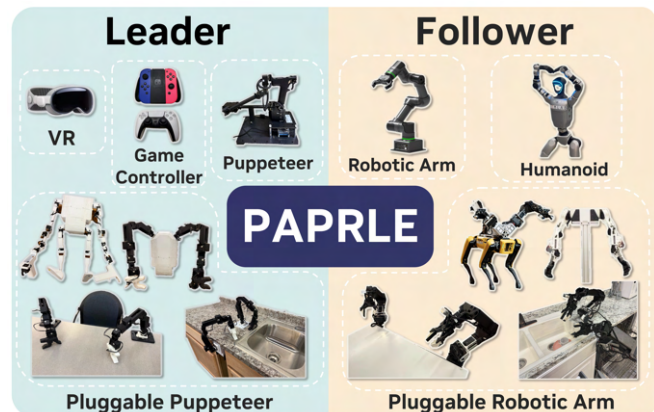
Fig. 1: Concept of PAPRLE. Various leader devices (left) can be flexibly paired with diverse robot embodiments (right) through a plug-and-play teleoperation system that supports modular and interchangeable components.
