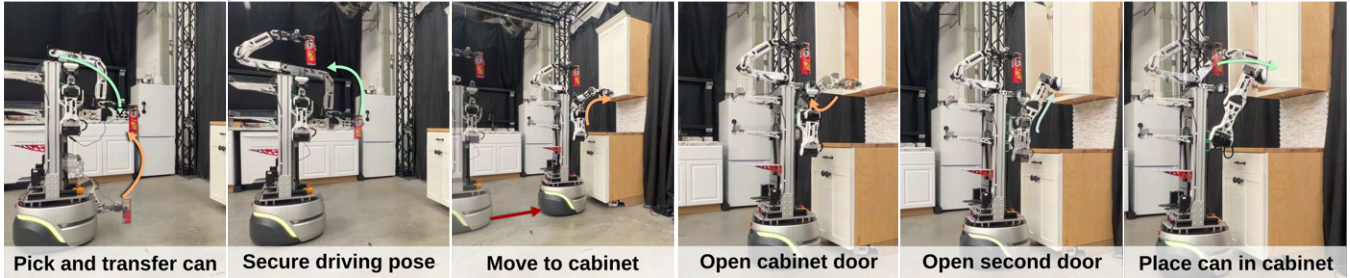
Fig. 8: Demonstration of the modularity of the proposed system. (Task one) MOMO utilizes a single arm on the neck mount to show its ability to extend the capabilities of a traditional serving robot by grasping, transporting, and placing an object without any human assistance. (Task two) Demonstrates how in the three-arm configuration, MOMO’s workspace is extended by grasping an obstruction off of the floor, handing it over to the arm on the neck mount, and then placing the obstruction on a shelf in a cabinet after opening the cabinet door.
