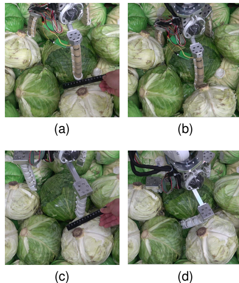
Fig. 18: Comparison of the performance between the previously developed hand in [10] ((a) and (b)) and the developed hand ((c) and (d)).
