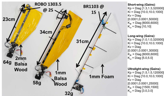
Fig. 8. SAM wings from left to right: short, long, ultralight; respective gains from top to bottom: short, long, ultralight.
