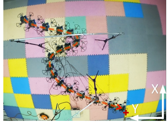
Fig. 11: Quadrotor robot experiment system setup (top view). A self-made quadrotor is powered via a cable connected to a ground power supply. It relies on the motion capture system (not shown) for localization and uses an onboard computer for high-level trajectory planning and a flight controller for low-level tracking. The task is to navigate the quadrotor from the starting position (upper-left) to the goal position (bottom-right red plus sign) while flying through two gates (formed by the vertical pole and two tripods) sequentially.
