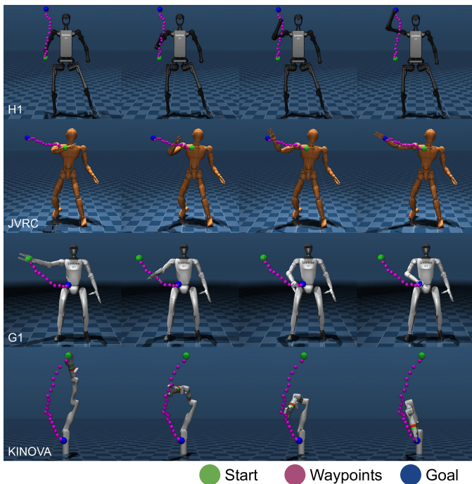
Fig. 5: Latent-Space Multi-Robot Control. A single policy controls the latent space to enable each robot to reach arbitrary goal positions (blue) from various starting poses (green). Intermediate waypoints along the generated trajectories are shown in purple.
