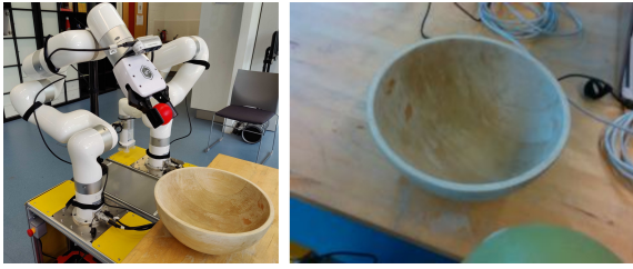
Fig. 6: Experiment setup of the object placing task (left) and typical wrist camera view (right)
