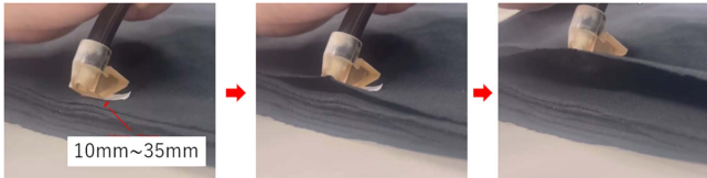
Fig. 12. Experiment of Drawing up single fabric edge by suction (suction of a single layer of fabric from a pile, with the fabric material being cotton and a thickness of 0.5 mm).
