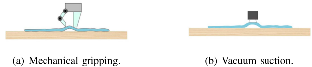
Fig. 3. Various methods to grasp flat-lying clothes. (a) Utilizing mechanical fingers to grasp flat-lying clothes (b) Employing suction pad to lift flat-lying clothes.
