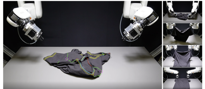
Fig. 1. T-shirt unfolding strategy based on seam features constructed from seam line segments and their crossings. The candidates for a pair of grasping points for a robot motion primitive are limited to the seam features marked in the figure.
