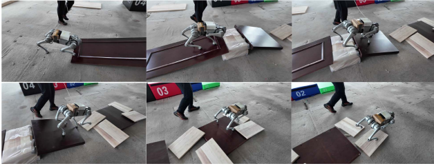
Fig. 15. Our RL+WBC framework enables the robot traversing diverse challenging terrains including slopes, obstacles, and uneven ground.
