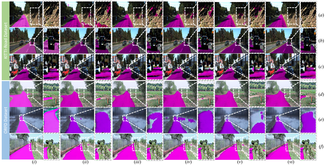
Fig. 3. Examples of TerrFlat-Seg results on the KITTI-Road and ORFD dataset with respect to different geometric inputs: (i) Ground-truth; (ii) Depth; (iii) Transformed disparity; (iv) HHA; (v) Surface normal; (vi) TerrFlat (Ours). (a)–(f) illustrate various challenging scenarios: (a) a road scene with sloped surroundings; (b–c) distant vehicles under complex illumination; (d) an unstructured muddy off-road terrain; (e) a snowy environment with strong reflectance; (f) a suburban road with irregular boundaries.
