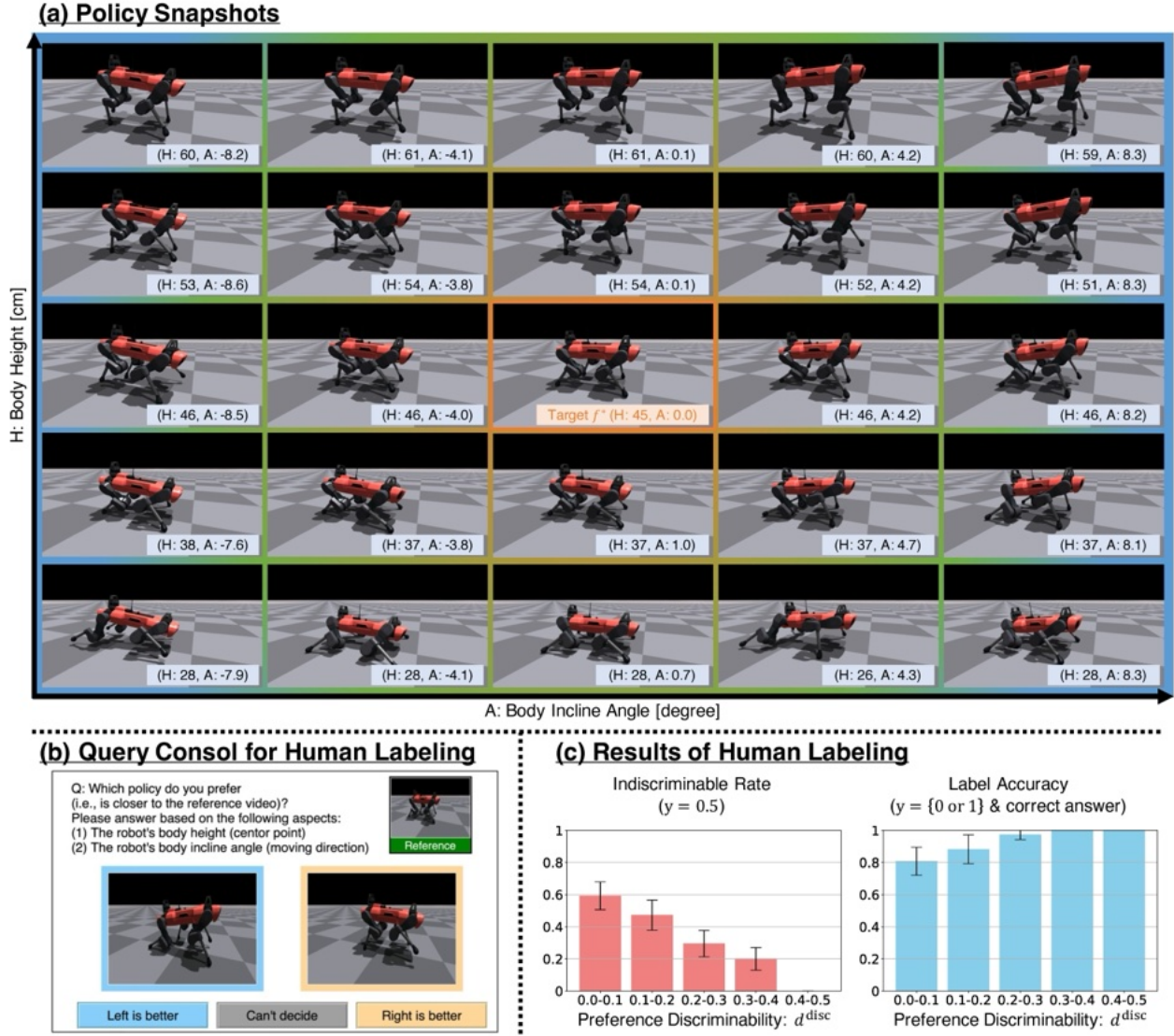
Fig. 3: Analysis of actual human query responses for determining the threshold of preference discriminability d^{disc} in the simulated annotator model: A questionnaire was conducted using a console system, as shown in (b). At the top of the screen, a reference video was displayed, showing a policy that matched a predefined target behavior. Below the reference video, two candidate policy videos were shown for comparison. Participants were asked to choose the trajectory closer to the reference by selecting one of three options: “Left is better”, “Right is better”, or “Can’t decide”. The candidate policies were prepared by exhaustively combining the listed values of Body Height [cm] \in \{29, 37, 45, 53, 61\} and Body Incline Angle [degree] \in \{-8, -4, 0, 4, 8\} . For each combination of these parameters, a policy was trained using DAPPER under an idealized setting where d^{disc} = 0 , by optimizing the behavior to match the specified Body Height and Body Incline Angle values until convergence. Participants were instructed to compare only two features defined by f^* : Body Height and Body Incline Angle. Gait patterns were excluded. They could prioritize the features freely, but were told to consider both. Policy pairs were sampled from (a), and 105 predefined queries were presented sequentially. The queries were selected to ensure diversity in preference discriminability d^{disc} . All participants evaluated the same set of queries, and the order of the queries was randomized for each participant. The results shown in (c) represent the mean and standard deviation across five participants.
