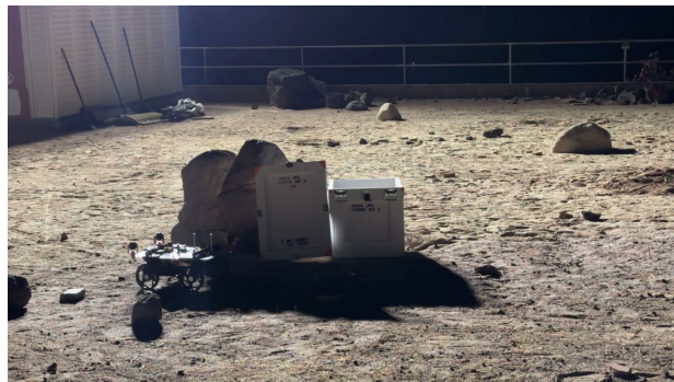
FIGURE 24. Nighttime testing conducted at the JPL Mars Yard exposed issues with shadows and the subsequent effect of creating large unknown regions for the Local Planner to treat as an obstacle.
