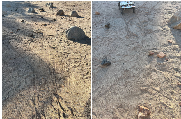
FIGURE 23. Long drives of up to 15 m in CFA-specification terrains to test long-horizon planning performance in aggressively cluttered terrain. The rover was able to successfully navigate many of these terrains. However, local minima such as box-canyon solutions shown to the right are possible without a sophisticated global initialization strategy.
