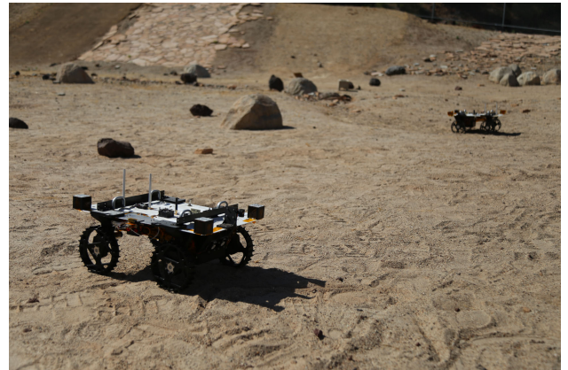
FIGURE 10. CADRE engineering model rovers driving in formation side-by-side during outdoor tests in the JPL Mars Yard. The engineering models for the CADRE mission allowed for extensive testing in outdoor environments and served as representative analogs for the flight rovers. Note wheel tracks traversed using CRESCENT.
