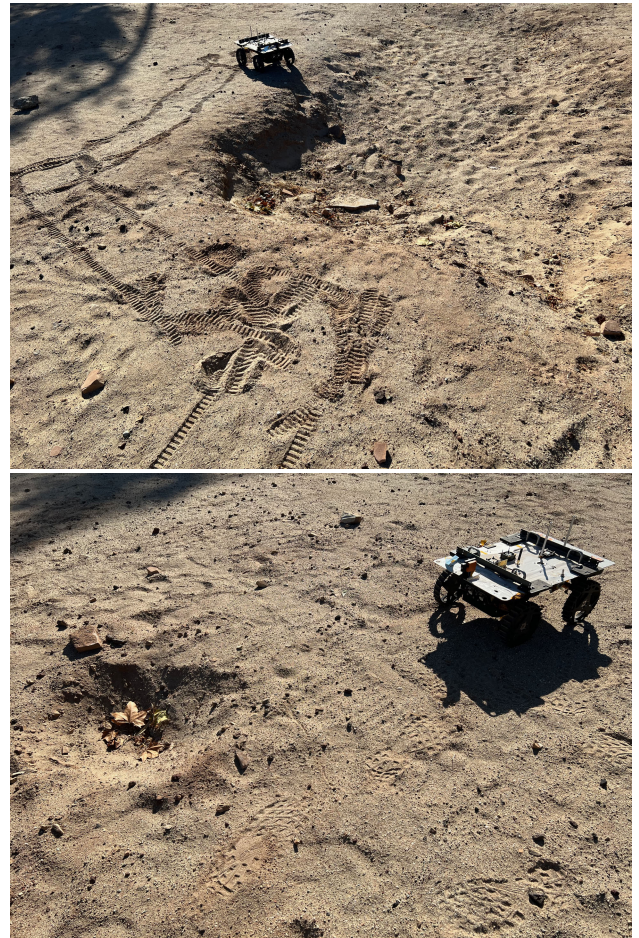
FIGURE 22. Testing was conducted to evaluate the efficacy of the planner in the presence of negative obstacles. A divert around a wide crater ( r > 2 m) is shown at the top; a smaller crater ( r \approx 10 cm) is shown at the bottom.
