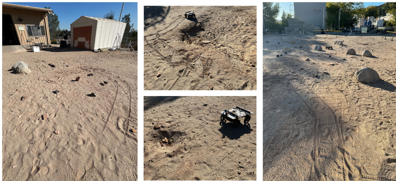
FIGURE 17. Planner was evaluated over case study and representative terrains in the JPL Mars Yard on engineering model hardware of CADRE flight units. Terrains included narrow and cluttered environments (left), craters (center), and approximate terrain specification environments (right).
