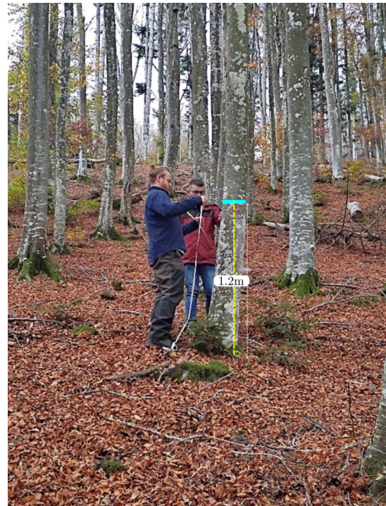
Fig. 4. Diameter at Breast Height (DBH) is commonly measured by expert personnel at 1.2 meters above the ground using a common tape measure.
