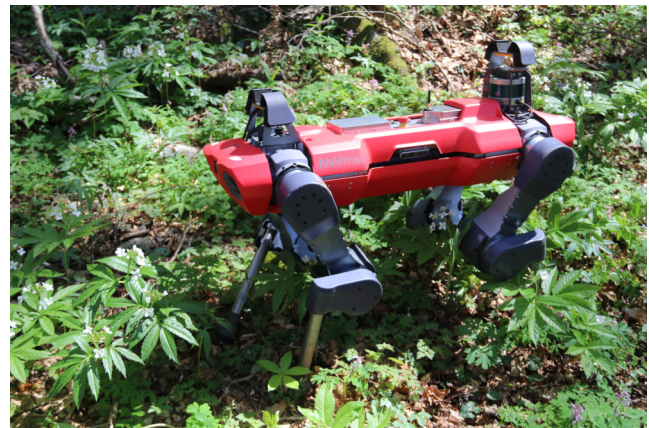
Fig. 3. ANYmal-C is a quadrupedal robot equipped with cameras, depth sensors and a LiDAR, enabling it to autonomously locomote in rugged, unstructured environments.
