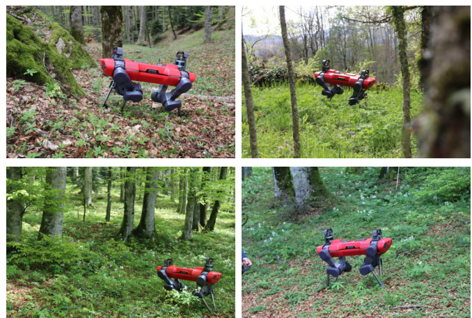
Fig. 6. The forest of Chiusi della Verna (Arezzo, Italy) represents an unstructured and harsh environment, with steep hills, branches and uneven terrain. Despite this, the quadrupedal robot ANYmal-C is able to locomote safely in this scenario.
