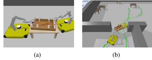
Fig. 6: (a) Validation of grasp configuration pairs for collective object transport in PyBullet. (b) Trajectory generation for a selected grasp configuration pair using the trajectory planner.
