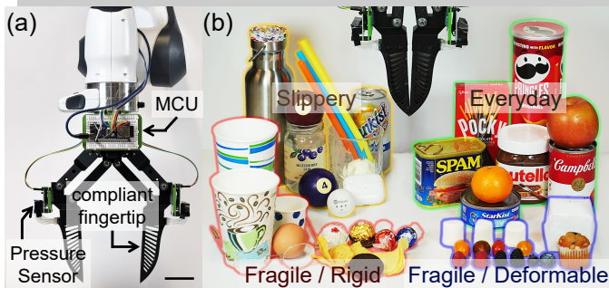
Fig. 5. Experimental Setup (a) FORTE is mounted on a Franka Emika Panda robot arm for table-top grasping tests. Scale bar represents 5 cm. (b) Objects used for evaluation. Fragile objects are selected to evaluate force estimation accuracy and gripper compliance, while slippery items and eight everyday YCB objects are chosen to assess slip detection performance.
