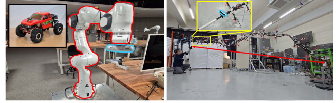
Fig. 7. Real-world experiment setup: The teleoperated robotic arm (Franka Emika Panda) is equipped with an RGB-D camera to reconstruct an RC car (left). 5-meter modular aerial robot is equipped with a front-mounted RGB-D camera to reconstruct the target valve (right). .
