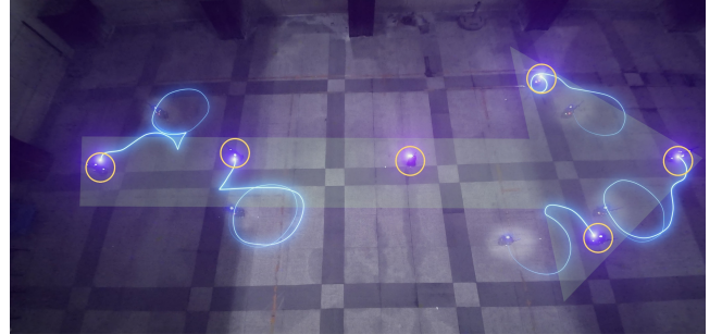
Fig. 1. Trajectories of a swarm of six robots forming an arrow shape in an external localization system denied environment. Each robot is equipped with an onboard light. This photo is obtained by long-exposure photography.
