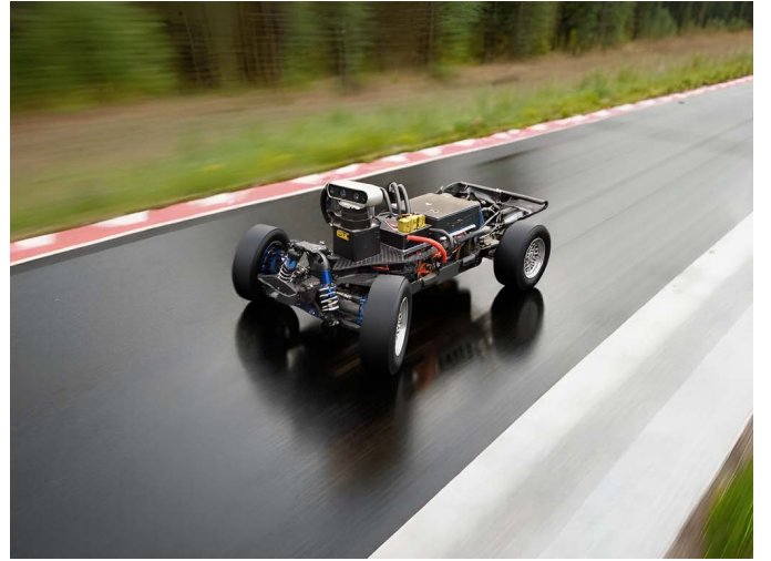
Fig. 1. The 1/10-scale race car prototype adopted in this study. The vehicle utilizes an ego-centric depth camera for perception of the environment. The policy processes depth images and proprioceptive states, then outputs commands to the electronic speed controller for motion control of the vehicle.
