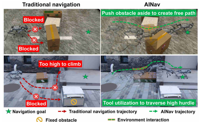
Fig. 1: Interactive navigation in challenging environments. In contrast to conventional obstacle-avoidance navigation systems that passively adapt to predefined free space and fail to reach goals in environments without feasible paths, AINav can push aside obstacles to create pathways within congested obstacles or utilize obstacles as tools to traverse excessively high hurdles, enabling interactive navigation in challenging environments.
