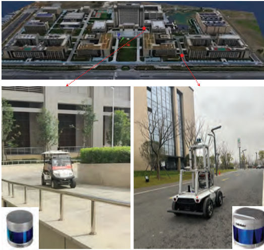
Fig. 10. Experimental setup for the self-recorded dataset. In particular, the top figure depicts the experimental setting, which is representative of a typical campus environment. In addition, the bottom two figures show two dataset collection platforms, 204AKZ (Eagle) and FR-09 (YUHESEN), equipped with two different LiDAR sensors, named VLP-32C (Velodyne) and Pandar40P (HESAI), respectively.
