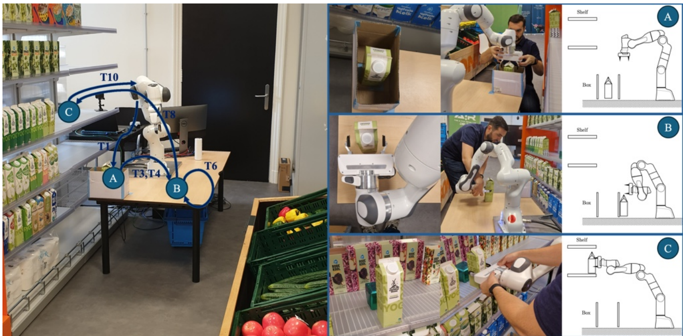
Fig. 2. Restocking task. A) Initial state, carton in the box, B) Intermediate placement for re-grasping, C) Final state, carton on the shelf.
