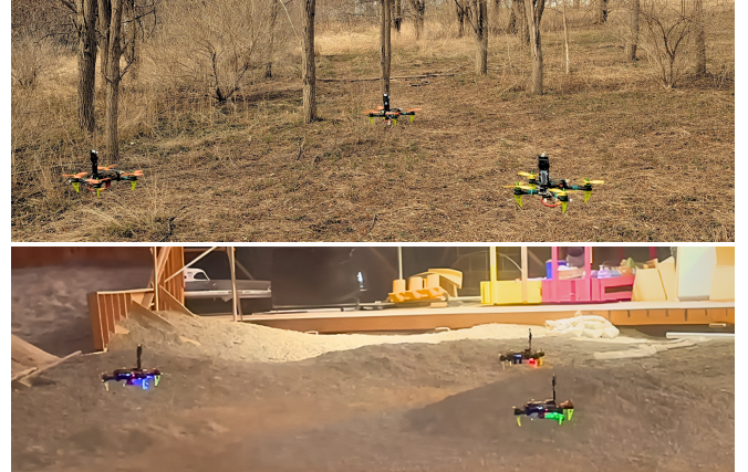
Fig. 1: A snapshot of three micro aerial vehicles (MAVs) flying in a triangular formation under a tree canopy (top) and in a GPS-denied environment inside a metal dome (bottom) using our proposed method for localization and distance-based formation control. All estimation and control is done onboard the MAVs in a decentralized manner. A video of all the experiments can be found at following link: http://tiny.cc/mara_loc_nav .
