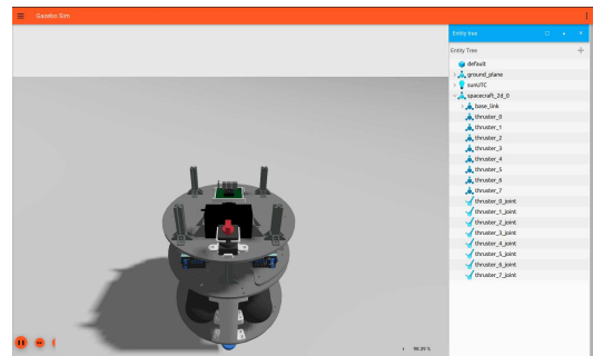
FIGURE 16: SITL simulation in Gazebo. The simulated model interacts with the PX4Space SITL setup and allows interaction with any of the control interfaces of the real platform, as well as simulating any of the radio-controlled flight modes.
