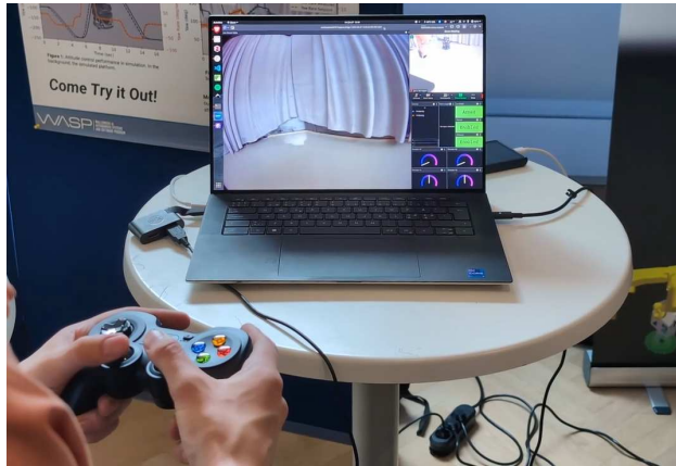
(b) A user operates the platform remotely. FleetMQ creates a peer-to-peer connection with minimal latency.
