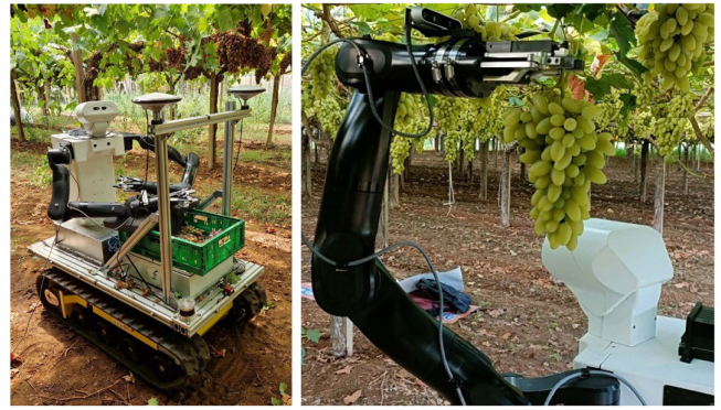
Fig. 1. The table grape harvesting robot equipped with an Intel RealSense D435i camera on the wrist.
