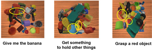
Fig. 3. Examples of simulated cluttered scenes with diverse language instructions in simulated environments.
