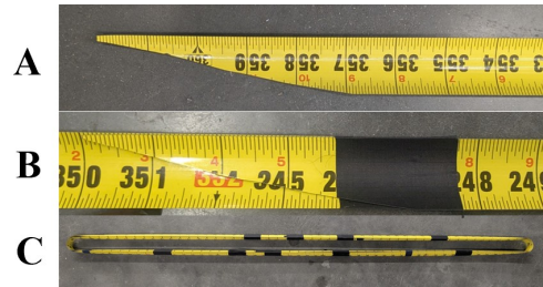
Fig. 5. Assembly process of tape spring with (A) 12.5 cm tapered cut at each end, (B) taper ends are joined using spinnaker tape, and (C) final tape spring
