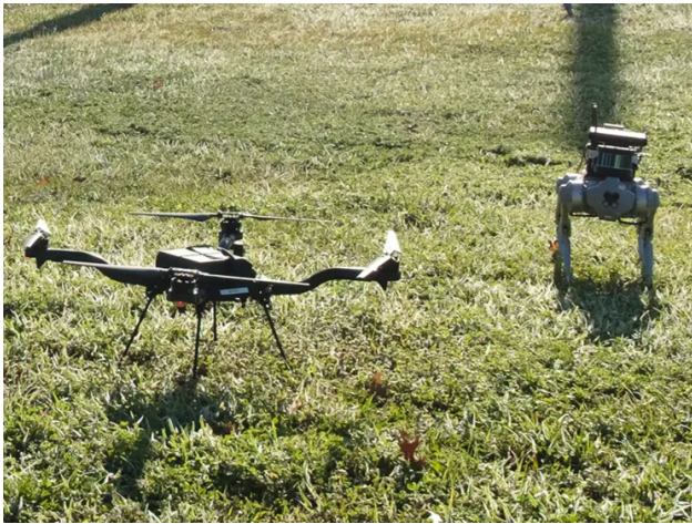
Figure 4. The Freefly Astro quadcopter (left) was used as the pursuer agent and the Unitree Go1 quadruped (right) was used as the target agent. The quadruped uses an Emlid RS+ RTK GPS for precise position updates, which is fused with attitude and heading data from a Microstrain 3DM-GX5-AHRS using the ROS2 robot – localization package.
