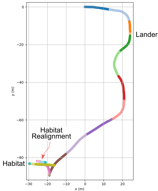
FIGURE 13. Eighteen path segments were executed during the semi-autonomous driving portion of the mission. These segments were recorded to create the smooth teaching path that was repeated afterward. Note that segments are short during precise alignments.
