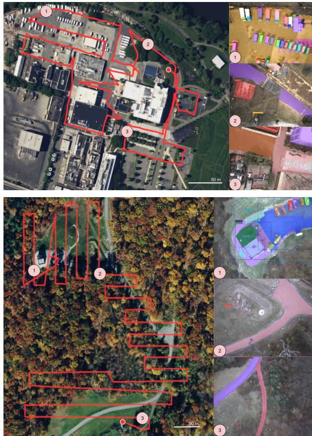
FIGURE 7. Example images of the detection and segmentation onboard the aerial robot. Top: Pennovation. Bottom: Range 15. The red line indicates the flight path of the UAV overlaid on Mapbox [79] satellite imagery.
