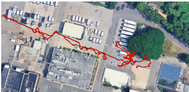
FIGURE A.6. UGV trajectory from the first system demonstration. Using the UAV-generated graph, the UGV travels over 700 m while finding objects and describing regions of the environment.
