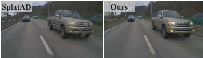
Fig. 9. Qualitative comparison of image rendering on our highway dataset. LiHi-GS produces sharper and cleaner reconstructions of moving vehicles compared to the blurry results of SplatAD, demonstrating the effectiveness of decoupled camera-LiDAR pose optimization for moving actor reconstruction.
