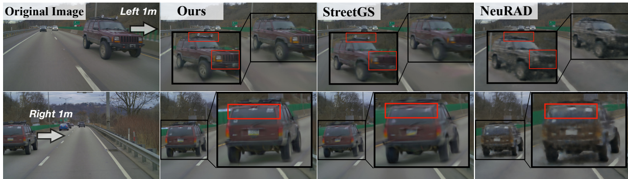
Fig. 12. Scene editing with lateral actor shift. LiHi-GS has the best overall image quality, given the accurate geometry learned from LiDAR supervision.
