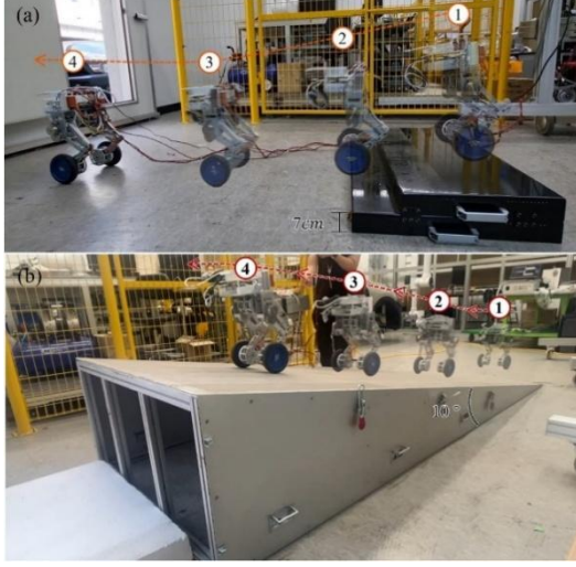
Fig. 2. Locomotive abilities on (a) a 2-step stair and (b) slope with a 10^\circ inclination.
