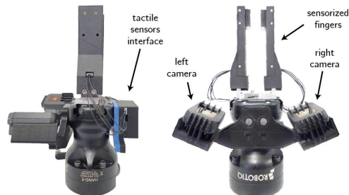
Fig. 2. Mechatronic tool for connector assembly comprising a converging stereo-based camera system and sensorized fingers.
