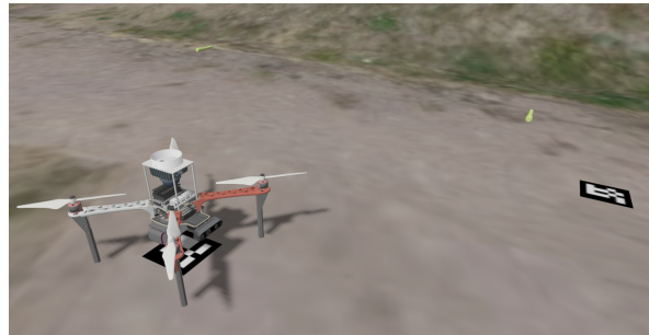
Fig. 1: Gazebo simulation environment showing the UAV and three experimental probes for localization and precision landing.
